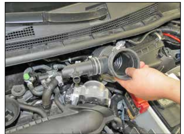
5. Remove the intake hose from the vehicle.
