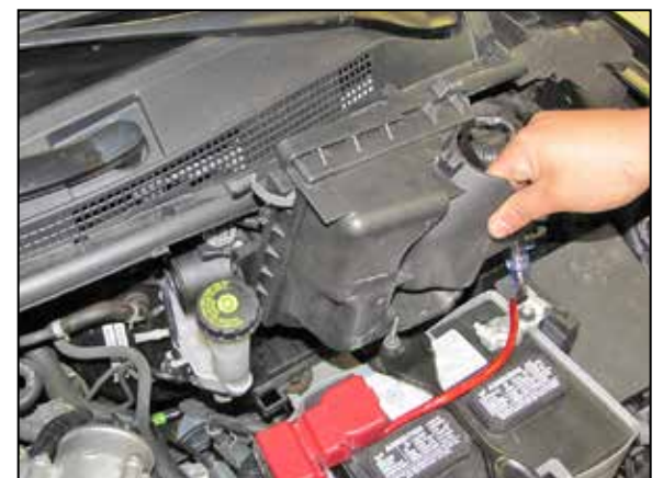
6. Release the two air box clips and then remove the front half of the air box and air filter.
