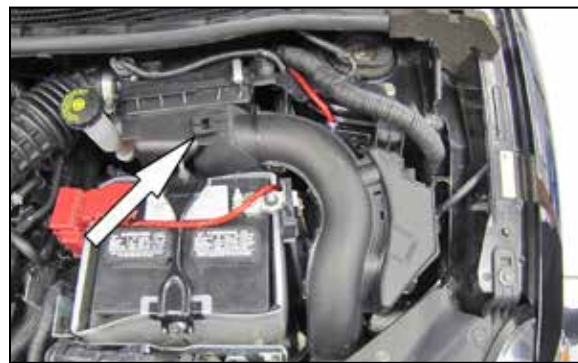
3. Unclip the fresh air intake from the air box and then pull the duct up to unhook it from retaining grommet and remove it from the vehicle.
