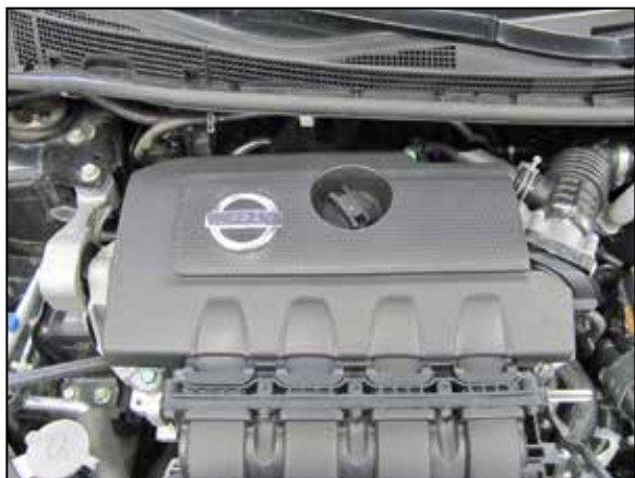
2. Lift up and remove the engine cover.
